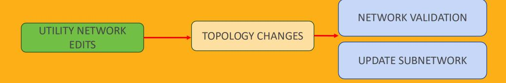
Usually covered as a part of updaters workflow but if you are receiving topology affecting data from External Sources like SCADA, ADMS or field workers you might could trigger a FME workspace to Validate Network and Update Subnetworks.
